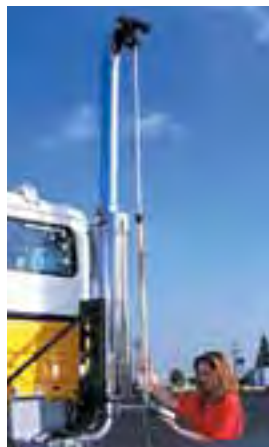
One person can run the entire test, even in the wind, since the sensor measures smoke inside the stack.
