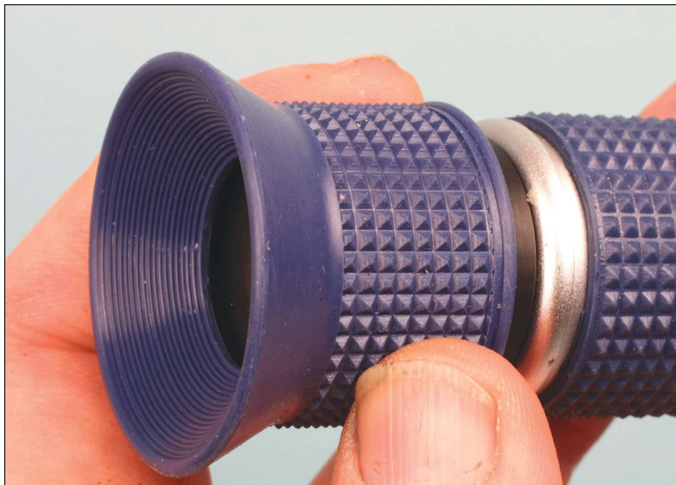
Diopter adjustment is handled by rotating the eyepiece to suit your eye.
