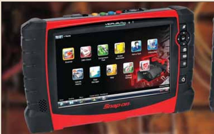
the freedom to work from anywhere in the bay. An internal hard drive allows you to store vehicle records, diagnostic data, test results and screen images, plus add your own software applications. The "S" button instantly captures screen images and provides navigation shortcuts.
