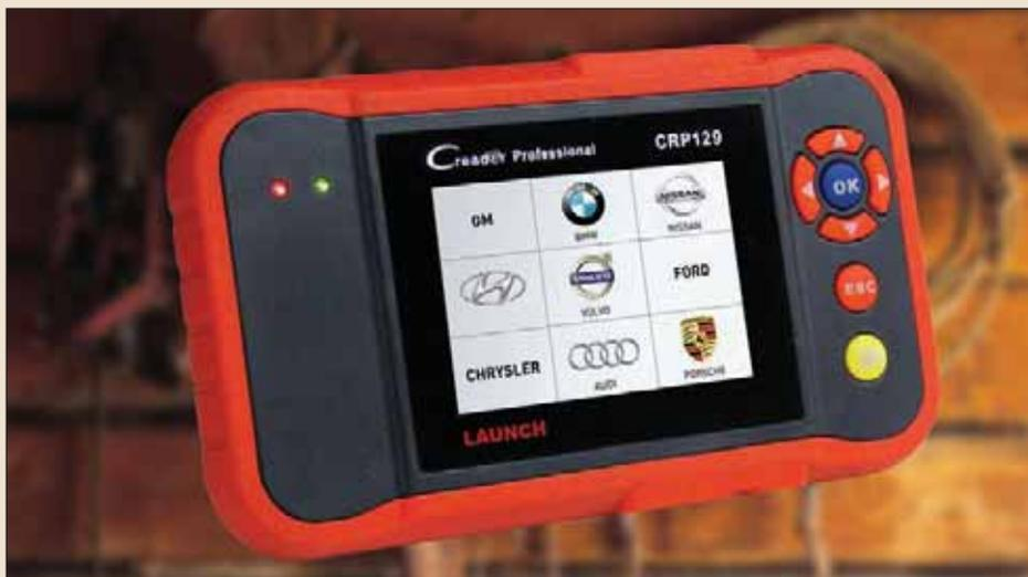
features include a 3.5-in. TFT color display, a lithium-ion battery, printing via PC, internet updatability and a rugged outer molding that protects the tool if it's accidentally dropped.
