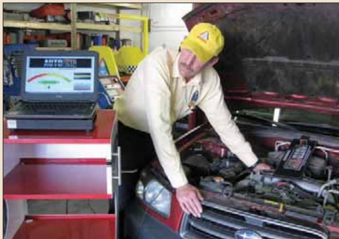
This led to the Auto EKG, a PC software system for combustion analysis, based on an existing tailpipe sensor that had been developed for misfire diagnosis by ATS (Automotive Test Solutions). AutoEKG software looks at the combustion efficiency by reading the pressure changes within
