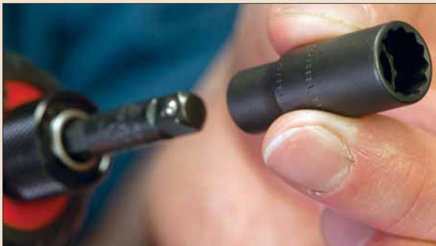
can take the flip socket to a number of other cars that use either screw head size on underbody pan fasteners—from Lexus, Infiniti and Mercedes-Benz, down to the Chevy Cruze/Buick Verano. The 12-point sockets engage every 30°, for better access.
