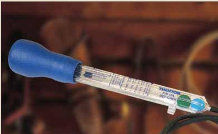
the number of floating discs indicates the urea concentration percentage (two should float if concentration is correct). The discs are temperature-compensating, so the DEF can be tested hot or cold. If the DEF is contaminated, a service procedure, such as flushing the tank with deionized water, is specified.
