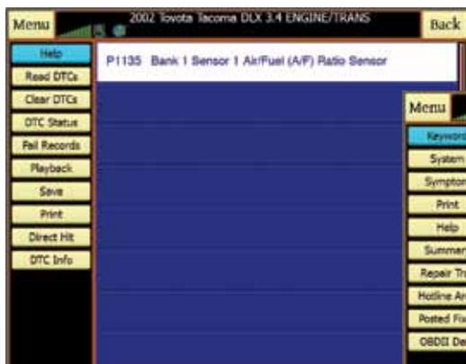
One button press of Direct-Hit Technician from the DTC screen sends the vehicle description and DTC to Identifix for an extensive search of their experienced-based information database.
