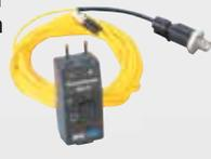
**No. 3500-03** – Surface temp probe - Measures surface temp of hoses, engine blocks, catalytic converters, and tire temp. K-type connector.
