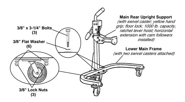
Note: The number of parts included in the Wheel Mate assembly kit are identified in parenthesis on the illustrations. Parts not identified with a number are single units.
