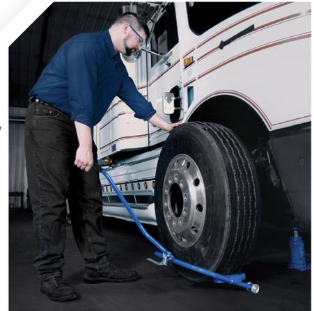
Clever Lever's easy lift and pull action removes the tire. Inside wheels pull off just as easy.
