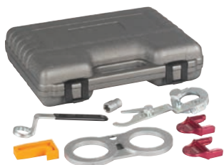
6687 GM 6 Cylinder Cam Tool Set • Required tools to adjust and hold cam shaft timing on GM 3.0 and 3.2 V-6 engines. • Kit is designed to save shop time when servicing GM 3.0 and 3.2 V-6 engines.
