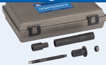
6918 Ford Spark Plug Remover Kit, 3V Engine • Unique design helps prevent breakage by locking the plug porcelain core to the plug hex allowing it to turn as one complete unit. • Will also pull plug porcelain core if plug hex only is removed. • Detailed Instructions to maximize success rate. Works on: • Ford 4.6L 3V V8 engines used in 2005–2008 Mustang, 2006–2008 Explorer. • Ford 5.4L 3V V8 engines used in 2004–2008 F-Series, 2005–2008 Expedition, 2005–2008 Lincoln Navigator. • Ford 6.8L 3V V10 engines used in 2005–2008 F-Series 250-350-450.
