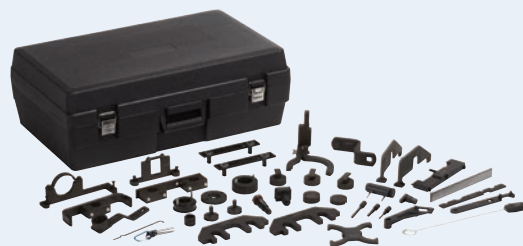
6690 Ford Master Cam Tool Kit • Contains 40 tools to ensure correct cam timing when servicing timing belts, chains, head gaskets, or other valve train repairs. • Covers L4, V6, V8, V10 engine with 2V, 3V, 4V valve configurations, model years 1991 – later. • Application guide with diagrams and blow molded case included.
