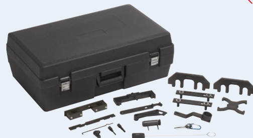
6690-1 Ford Cam Tool Kit Update • Contains 18 tools, with case locations for addition of the popular 6489 Ford Cam Tools, making a 6690 Kit. • Ford Cam Tools ensure correct cam timing when servicing timing belts, chains, head gaskets, or other valve train repairs. • 6690-1 tools cover L4, V6, V8, V10 engines with 3V & 4V valve configurations, model years 2004 – later. • Application guide with diagrams and blow molded case included.
