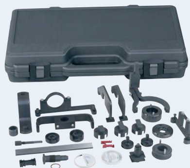
6489 Ford Cam Tool Kit • Ensure proper cam timing when you replace a head gasket, replace a timing belt or chain, or complete any valve train repair. • The 22 tools in this Master Kit covers 1992 through 2012 applications and comes in a molded storage case. Service the following engines: - 4.6L/5.4L/6.8L Modular; 3.8L V6 - 4.2L V6/5.0L V8; 3.0L Taurus - Windstar; 4.0L V6 Aerostar - Ranger and Explorer - 2.0L DOHC Zetec
