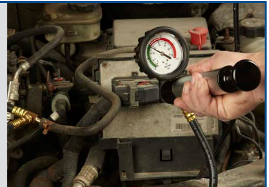
Connects to degas bottle to test caps, hoses and system pressure for leaks
