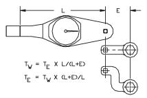
TW = Torque reading on wrench
