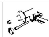
Hanger tube removal with No. 1743 set.
