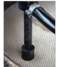
Long nozzle with floating puck for standard open face DPFs.
