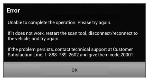
The Errors in AST/ASDTC will be made consistent and simple. The controller can either be read or it cannot. The error message for controllers that could not be scanned will be changed to "This vehicle may be missing optional equipment. This controller may not be available, or there may be a communication problem."
