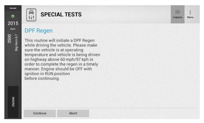
Manual DPF Regeneration – Forces the Regeneration process to run when conditions are correct
