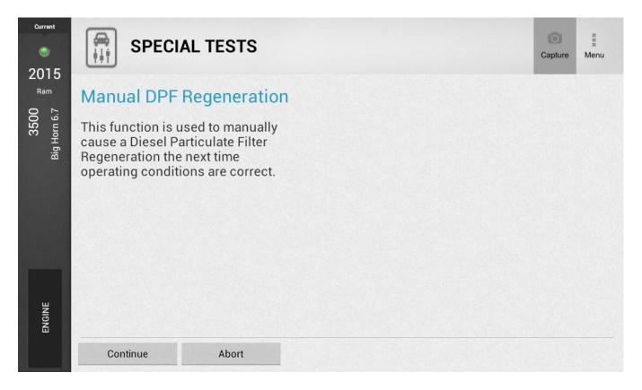
Manual DPF Regeneration - Allows user to reset the learned values after filter is replaced
