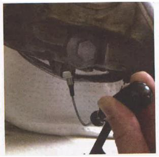
then using the proper size wrench broke the drain plug loose, attached the magnetic socket to the driver and unscrewed the plug until it came out. When it fell free of the crank case I thought, Darn!, but then I remembered it was still hooked to the socket. Cool! I cleaned up the drain plug, checking for metal fragments and it was ready to reinstall. After changing the oil filter, I replaced the drain plug and I was ready to fill the bike with oil and go riding.
