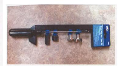
I have used the Drain Plug Pro several times since receiving it in the mail, but not just for the drain plug. I found it to be helpful in starting bolts that you can see but are hard to get your hand on (like the allen screws on the stereo unit inside the batwing fairing of an Ultra Classic).
