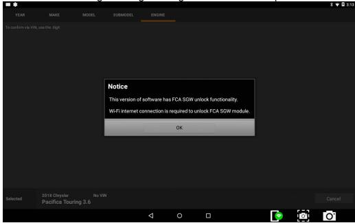
**Clearing DTCs** on FCA SGW enabled vehicles requires an internet connection in order to relay the details of your 2018 and newer FCA vehicle to an online service that can unlock the Gateway. Just connect to the internet, read DTCs and utilize the "Clear DTCs" button:
