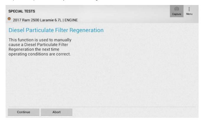
**DPF Reset Option** – Allows user to reset parameters used to schedule a DPF regeneration cycle to zero. Used after a DPF system component is replaced to reset system to zero for regeneration
