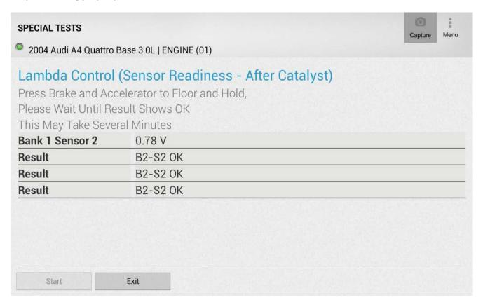
Lambda Control (Delta Lambda Bank 1/3) – Tests Bank 1/3 Sensors to make sure they are working properly
