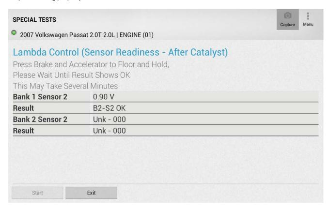
**Lambda Control (Sensor Exchange)** – Tests and compares Oxygen Sensors, after Catalytic Converter, to the Air Mass to make sure they are working properly
